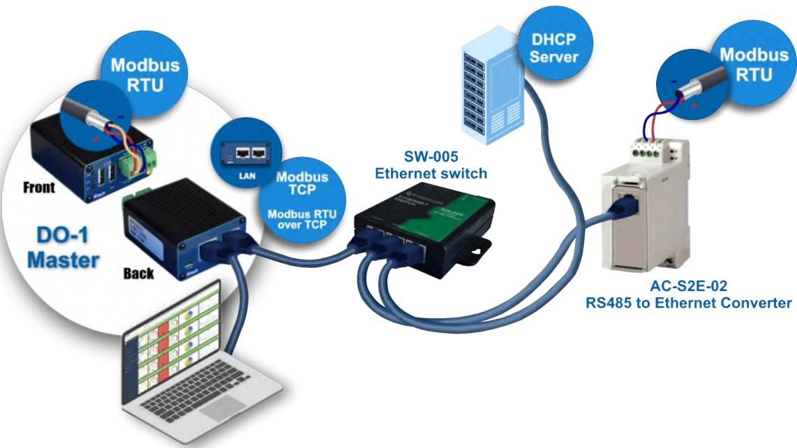
**Modbus RTU** is a serial communication protocol using mainly RS-485. With RS-485, the range can be up to 4000 feet (1200m) and the speed up to 115200 baud. At 115200 baud, the range is reduced. Devices can be daisy-chained with RS-485.
