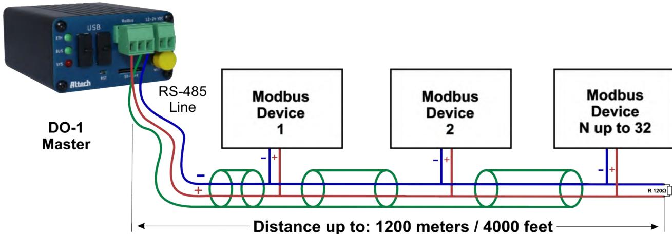
Reversing the 'A/+' and 'B/-' connections of a device not only stops communication between these devices, but also stops communication in the entire network of the system due to the incorrect DC (polarization) voltage of the terminals of the incorrectly connected device. To prevent this from happening, wires of the same color are used to connect one type of terminal (e.g. red for A/+ and blue for B/-).
