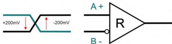
Voltage (A+) - Voltage (B-) => 200mVdc : Logic 0 | Voltage (B-) - Voltage (A+) => 200mVdc : Logic 1
