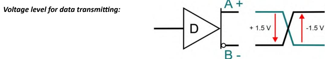
Voltage (A+) - Voltage (B-) => 1.5Vdc : Logic 0 | Voltage (B-) - Voltage (A+) => 1.5Vdc : Logic 1
