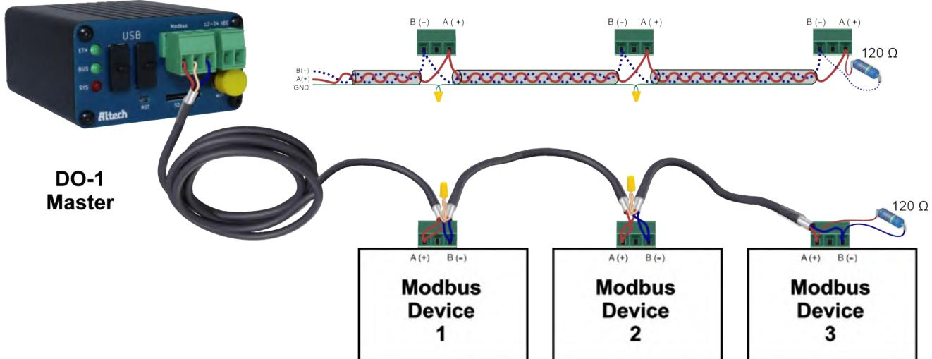
Note: The unshielded wires of the shielded cable should be kept as short as possible. It should also be noted that a secure connection of the cable shield to the Modbus devices is necessary to ensure proper shielding over the individual cable sections. This will ensure interference-free data transmission.
